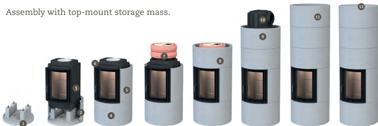
BSO 01 assembly steps. Only the most important assembly steps are shown.
