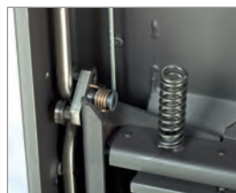
Opening the lifting door for cleaning with the “click-clack” mechanism.
