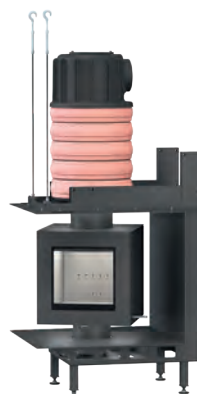
DF 33 with niche cladding 01 and attached storage mass MAS (in the case of static load on the mounting frame bracing the rear wall/ceiling is required).
